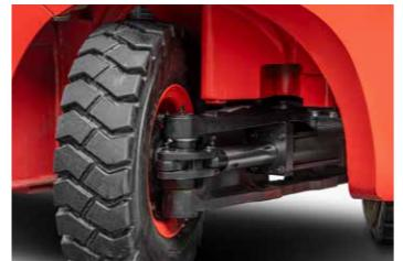
The steering axle is installed with rubber pad, which effectively improves the operation comfort and reliability.
