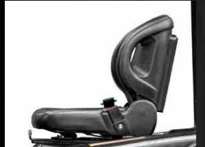
The truck comes standard with OPS system, and an optional adjustable speed limit function is available to enhance operational safety.
